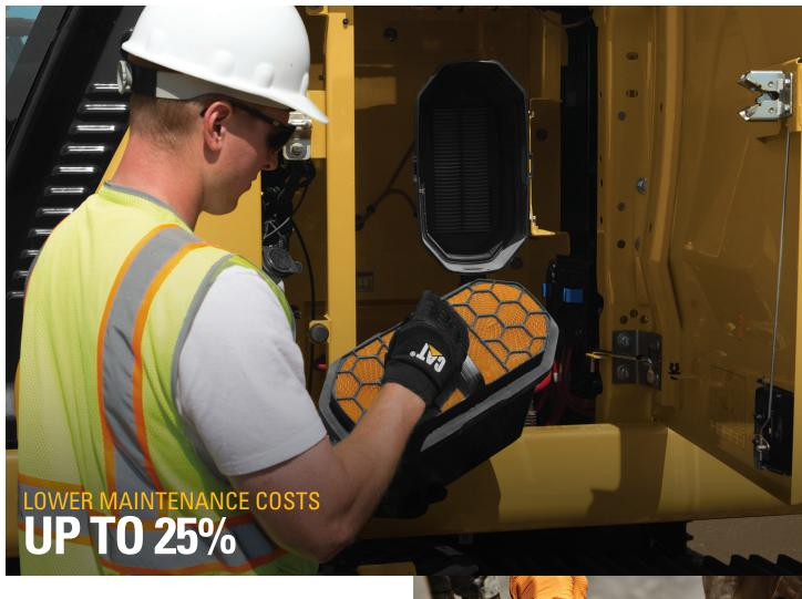
With extended and more synchronized maintenance intervals, you get more done at a lower cost compared to the 320F. Consolidated filter locations make service faster. Hydraulic, air, and fuel tank filters have increased capacity and longer life.
